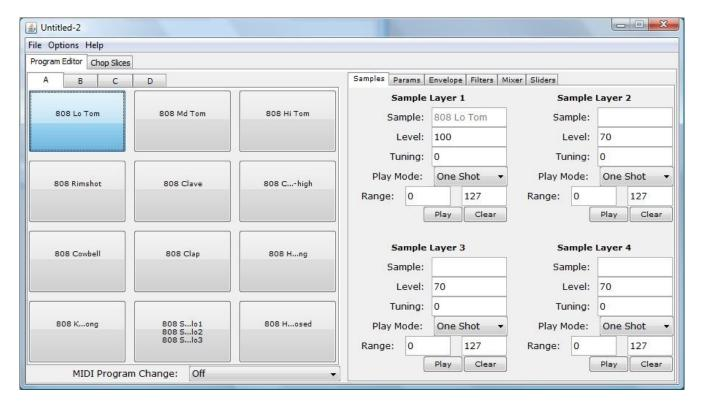
On the left half of the window there are the four banks of pads. Each pad shows the names of the samples assigned to it (zero to four samples per pad).
