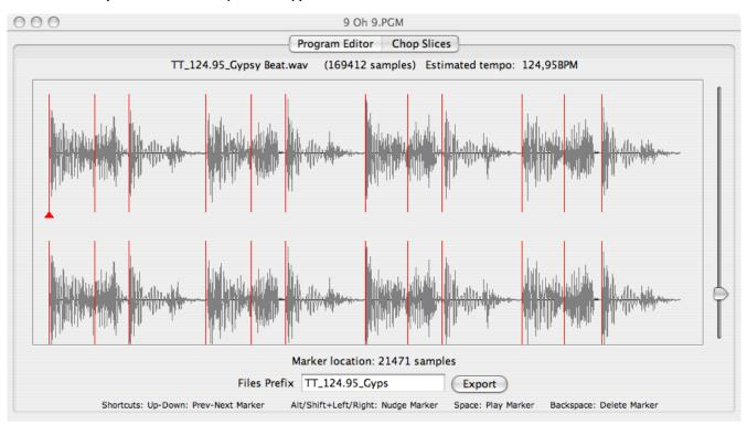
The editor seamlessly processes the file to detect every beat and marks them with red markers. The slider on the right is a sensitivity settings to help tweak the detection: just move it to see the changes.
